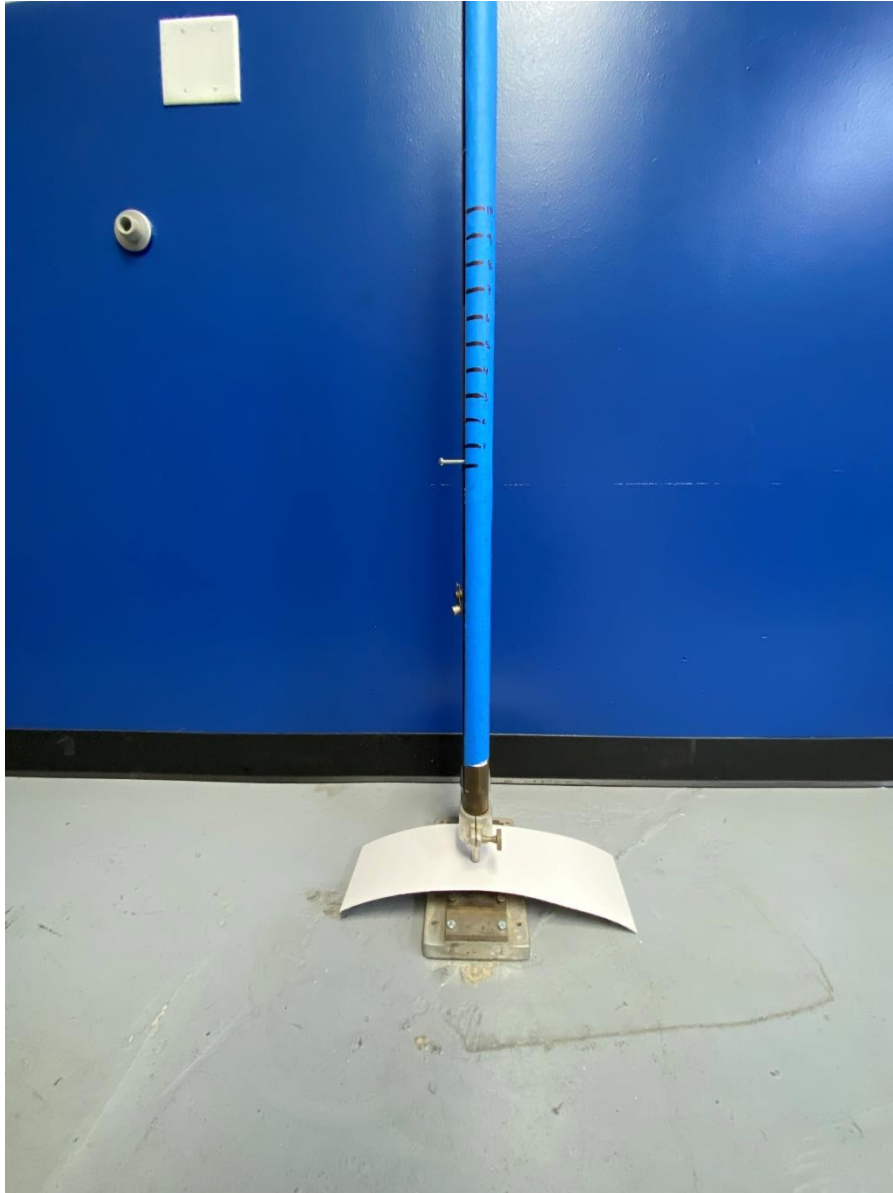
Photo 2: Impact Tester with configuration C.125 head
