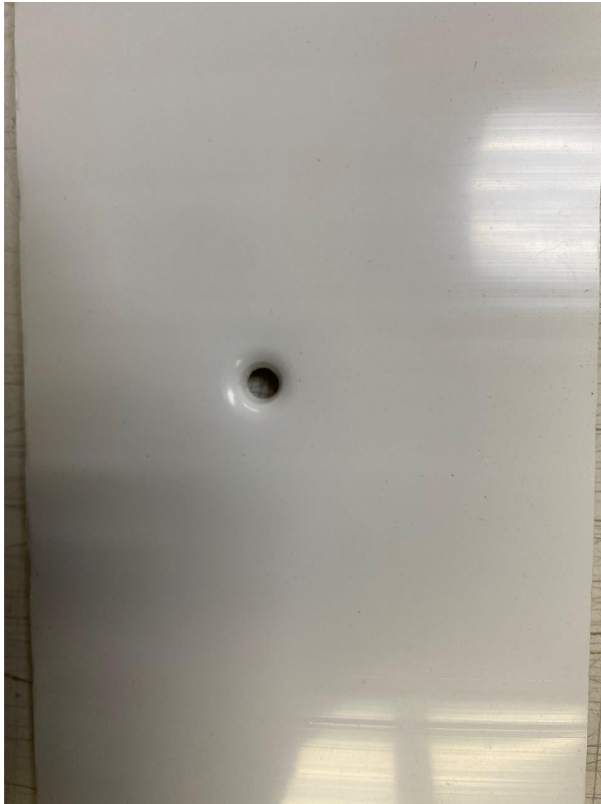
Photo 3: Typical Ductile Failure
